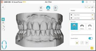
Add a base to your digital impression using Model, which can be used for 3D printing.\*
